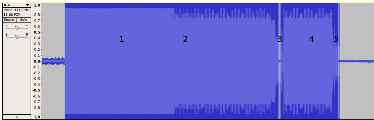
Figure 1: Waveform of sample program (1: 6 kHz lead-in; 2: 256 x 0xFF; 3: file header; 4: 128 x 0xFF; 5: data)
